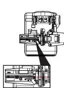
2. Place the fiber on the proper groove and check target length.
