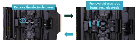
Clean the new electrodes with alcohol soaked clean gauze or lint-free tissue, and install them in the splicer.
