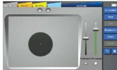
Testing fiber end face on connectors with FIBER MICROSCOPE is very important, because a polluted or damaged connector can cause critical damage to test results as well as testing port.
