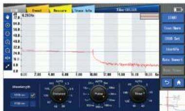
OTDR-mode enables you to measure distance, loss, reflectance, attenuation, ORL and sum on an optical fiber. When operating Auto-mode, test is automatically done without additional setting. The test results can be stored in 3 types of format (image, SOR, PDF)
