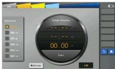
OPM (Optical Power Meter) is used for accurately measuring optical power on fiber optic networks operating at 850nm, 1300nm, 1310nm, 1490nm, 1550nm, 1610nm and 1625nm.
