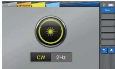
VFL (Visual Fault Locator) visually identifies the location of bending point, faulty connector or splicing point by emitting a bright red laser (it can reach a maximum of 10km), and this is a must function that workers need on the field.
