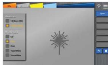
Invisible light source (1310/1550nm) can provide the following sources of light: CW, 1kHz, 2kHz modulated and 1kHz & 2kHz blink.
