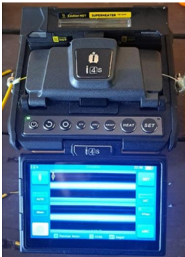
Fig.6. Fusion performed without arc calibration
